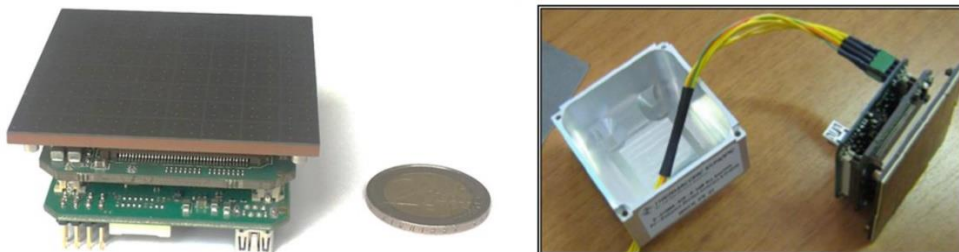
Figure 4: PDM front-end electronics consisting of SiPM tile, ASIC and FPGA boards. The PCBs are accommodated in an aluminum case by means of four through screws.
